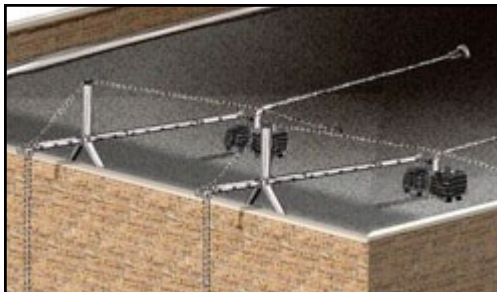
Outrigger beams with tiebacks and counterweights
